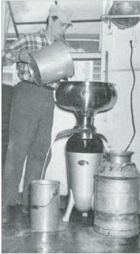
Cream separator powered by an electric motor.
