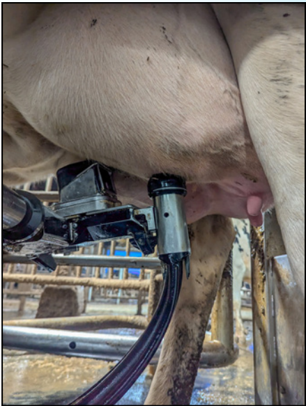
Ensure that teats are thoroughly cleaned before teat cups are attached, as shown.
