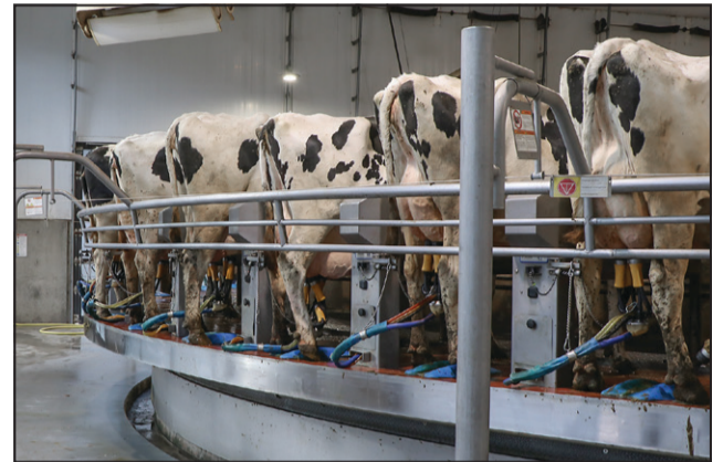
The 50-stall rotary allows for the entire 680-cow herd to be milked in roughly three hours at Bredale!
